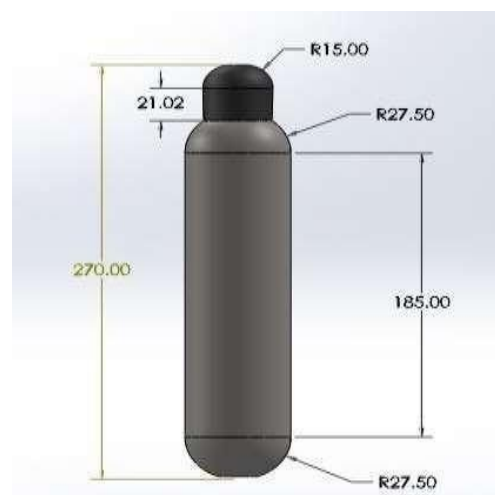
Figure 2: Cylindrical Accumulator with Dimensions
