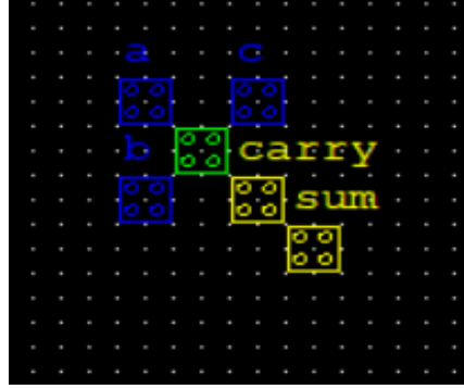
Figure 2: Proposed QCA Adder-2
