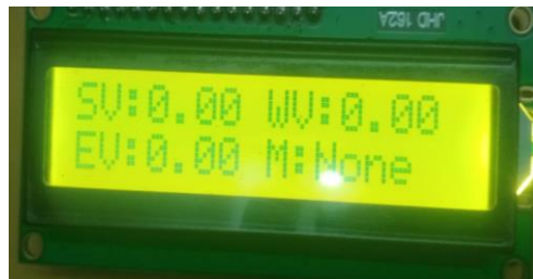
Figure 6(c): All Input Power Are Normal
